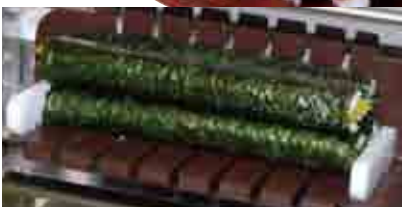
4 hosomaki (small roll) can be set on cutting table : 2,200 rolls / hr
